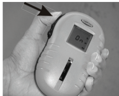
1. Press Power ON Turn Unit ON by pressing power button. Display will read "On"
